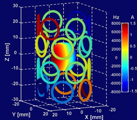
Figure 1: Theoretical coil setup. A total of 24 coils (15 turns, diameter 13 mm) was arranged in 4 rows with 6 coils each on a cylindrical surface (diameter 30 mm). The coils' color coding represents the current distribution to create a 10 kHz/cm X gradient in a centered, barrel-shaped 2.6 mL VOI for which the frequency distribution is coded in color.
