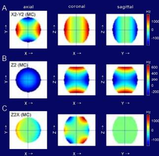
Figure 5: X2-Y2 (A), Z2 (B) and Z2X (C) terms at 1 kHz/cm<sup>2</sup> amplitude were generated with the MC approach at 980 mA, 434 mA and 783 mA maximum currents, respectively. The experimental field shapes resembled the theoretical target fields with a high degree of similarity ( $1-R^2 \leq 5 \cdot 10^{-3}$ ) and average deviations of the MC fields were  $\leq 1\%$ .
