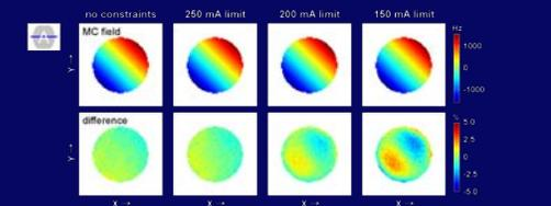
Figure 6: Experimental MC gradient generation of a 2 kHz/cm XY gradient field in a single slice of the barrel-shaped basic volume. Improved field accuracy was achieved for all current constraints when compared to the consideration of the whole barrel-shaped VOI (Fig. 4). For a given accuracy, these improvements directly transferred to strongly reduced maximal currents and improved gradient efficiencies.
