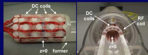
Figure 2: Experimental realization of the MC setup. Left: 24 individual coils were placed on a cylindrical former made of acrylic tube. The inner diameter of the former of 25 mm allowed the placement of a glass bottle or a mouse cradle inside the device. Right: Firm mounting of the former inside the RF resonator provided a close integration of both systems and allowed their simultaneous use.
